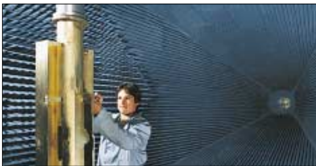
Full Size antenna section undergoing azimuth pattern test in one of two Andrew anechoic chambers dedicated to broadcast products.
