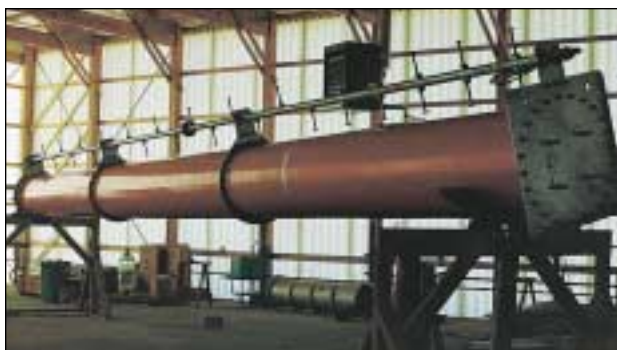
GUIDELINER antenna for WTIU channel 30 undergoing inspection.
